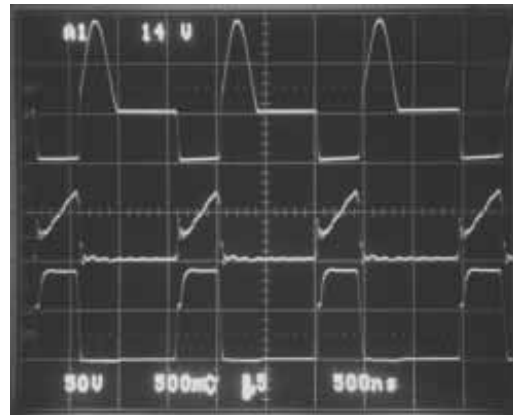
Top: V_{\text{DS}} @ 50 V/div Middle V_{\text{SENSE}} @ 500 mV/Div Bottom: V_{\text{GS}} @ 5 V/div Time: 500 ns/div
